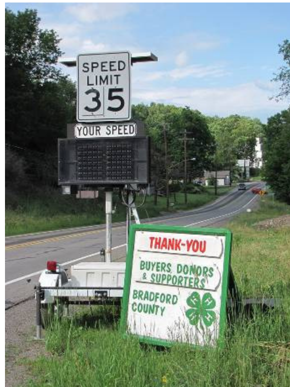
Figure 27: An example of a speed monitor trailer in Alba Borough.
